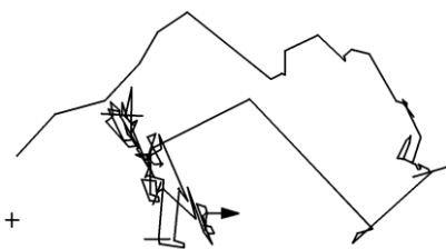
Fig. 6b. Projection of the Iris (4-4-3) learning trajectory trained with VSS in the third and fourth PCA direction. The cross shows the zero point in the weight space, and little bars separate the training epochs.
